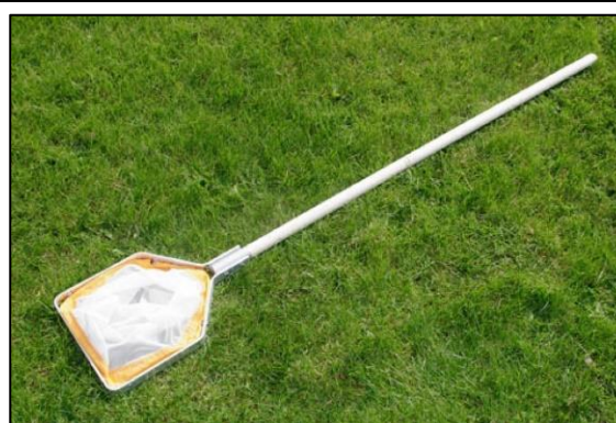
Figure 6-1. Standard hand net for sampling macroinvertebrates
